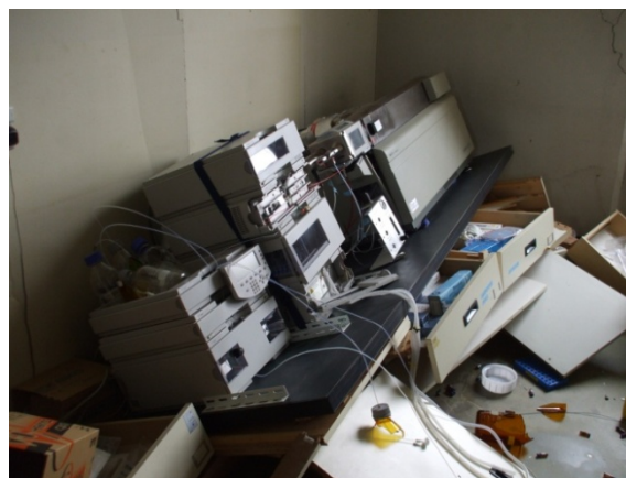
4階 LC/MS/MS 架台の脚が折れ本体破損
