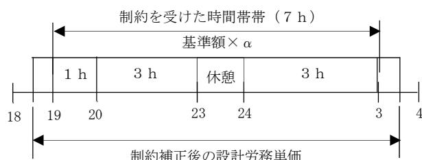
$$\begin{aligned}\text{設計労務単価} &= [\text{基準額} + \text{割増し賃金}] \times \text{補正割増し係数} \\ &= \text{基準額} \times 1.428 \times 1.14 \\ &= \text{基準額} \times 1.628 \\ \text{ただし, } \alpha &= \text{割増し率} \\ &= (1h \times 1.0 + 6h \times 1.5) / 7h \\ &= 1.428 \\ \text{割増し賃金} &= \text{基準額} \times 0.428\end{aligned}$$
