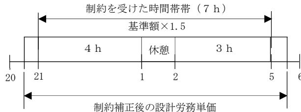
$$\begin{aligned}\text{設計労務単価} &= [\text{基準額} + \text{割増し賃金}] \times \text{補正割増し係数} \\ &= \text{基準額} \times 1.5 \times 1.14 \\ &= \text{基準額} \times 1.71 \\ \text{ただし, 割増し賃金} &= \text{基準額} \times 0.5\end{aligned}$$
